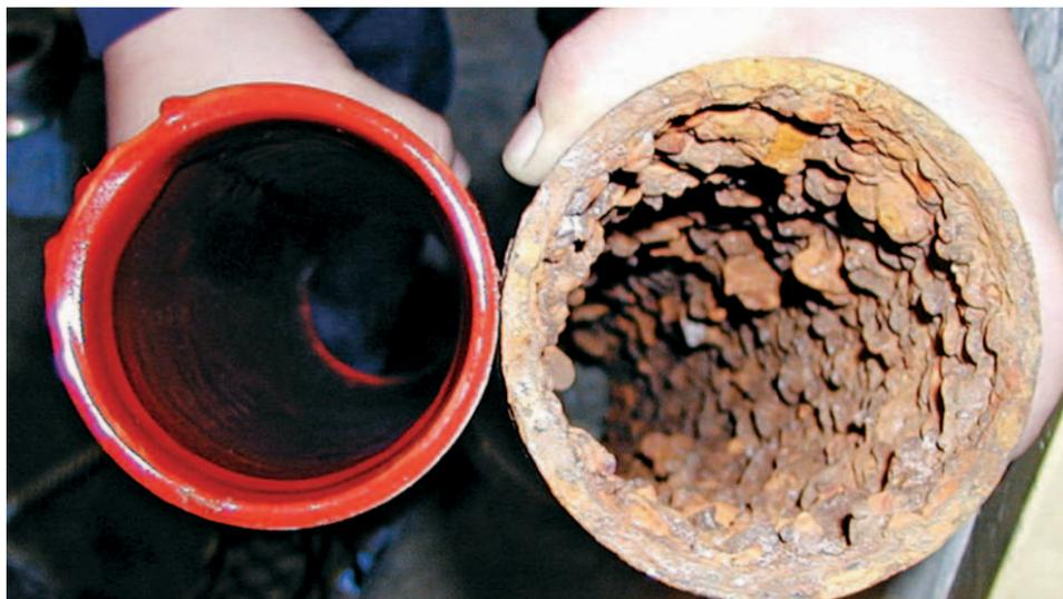
it once, and let it sit for 12 to 16 hours. The acid dissolves the scale and moves it out of the system," he says. "It doesn't just mask the odor." If buildup is severe, Leclerc suggests several applications spread over the course of a week. Hard-plumbed black-water lines in large yachts tend to build up scale throughout their length, requiring cleaner to be circulated throughout the system.
